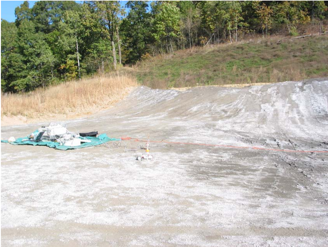
Figure 2-2 Mercury volatilization field measurements on barren ash
