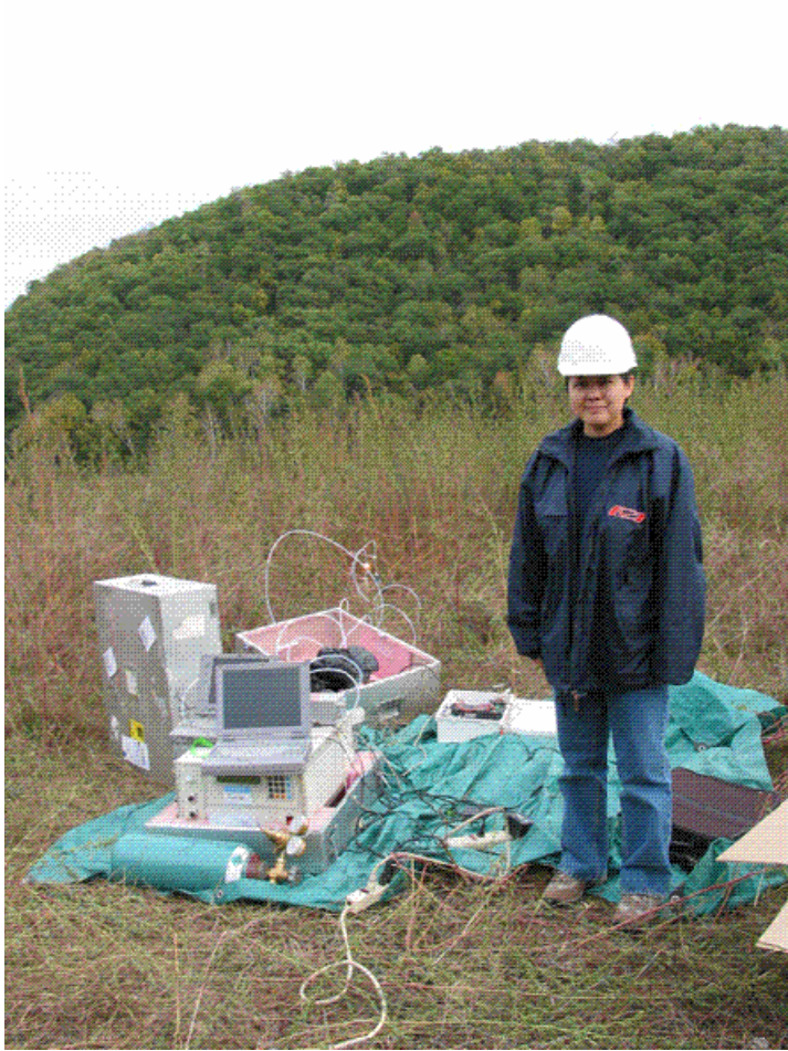
Figure 2-3 Mercury volatilization field measurements on vegetated ash
