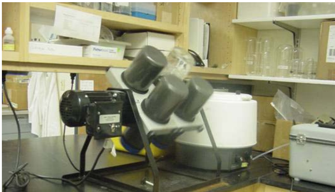
Figure A-7 SPLP Leaching Set-up
