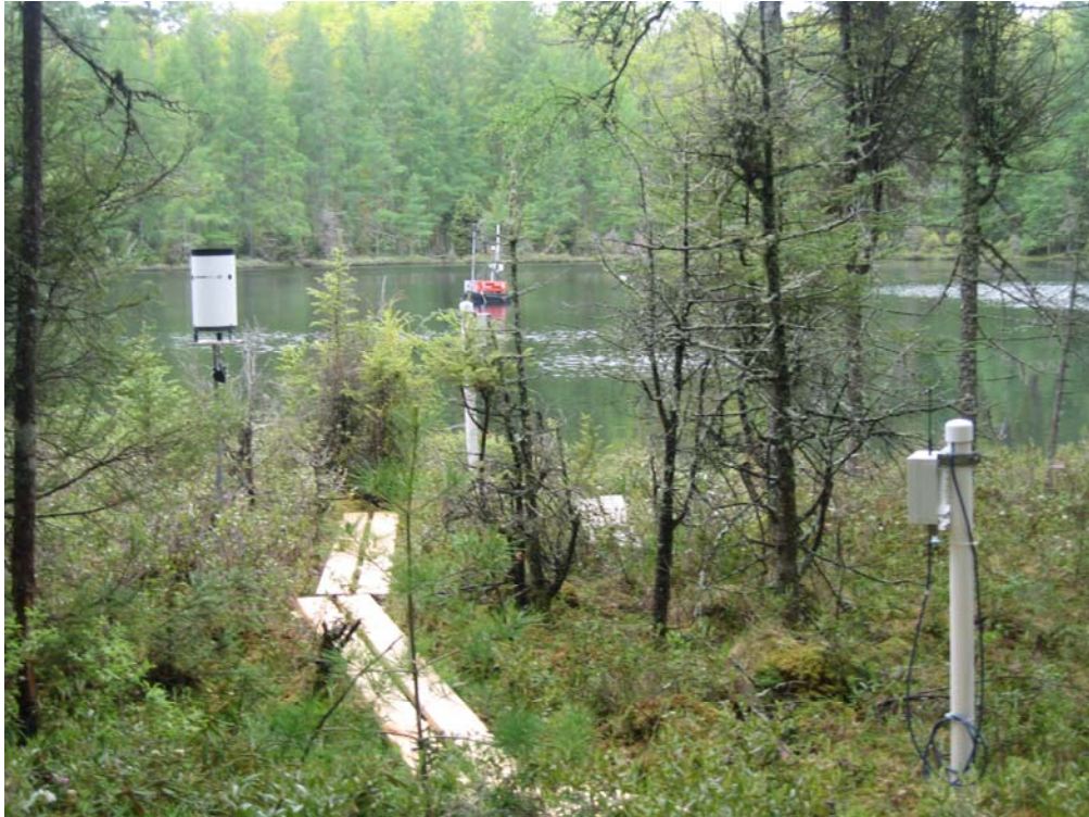
Figure 18. INW-based monitoring network in the TB catchment, showing two wetland wells and the rain gauge. Red object near center of lake is the GLEON buoy.
